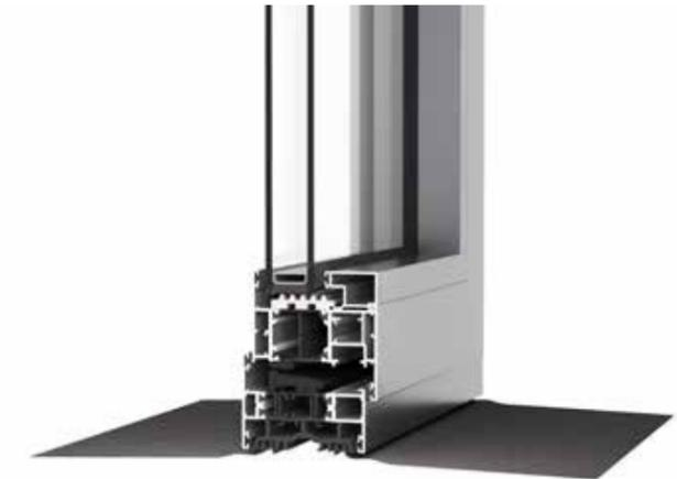
Universal EPDM carrier groove – allows clip-in EPDM strip and direct lug fixing to be used on all outer frames, frame extenders and sub cill profiles. The EPDM can be fitted reliably and easily with a 'snap-in' PVC profile, supplied by AluK.
